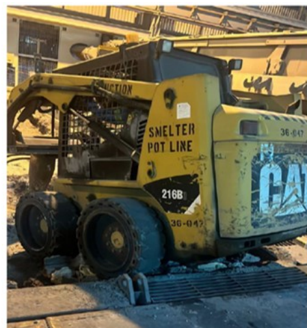
Figure 18. Use of bobcat to detach anode and metal.
