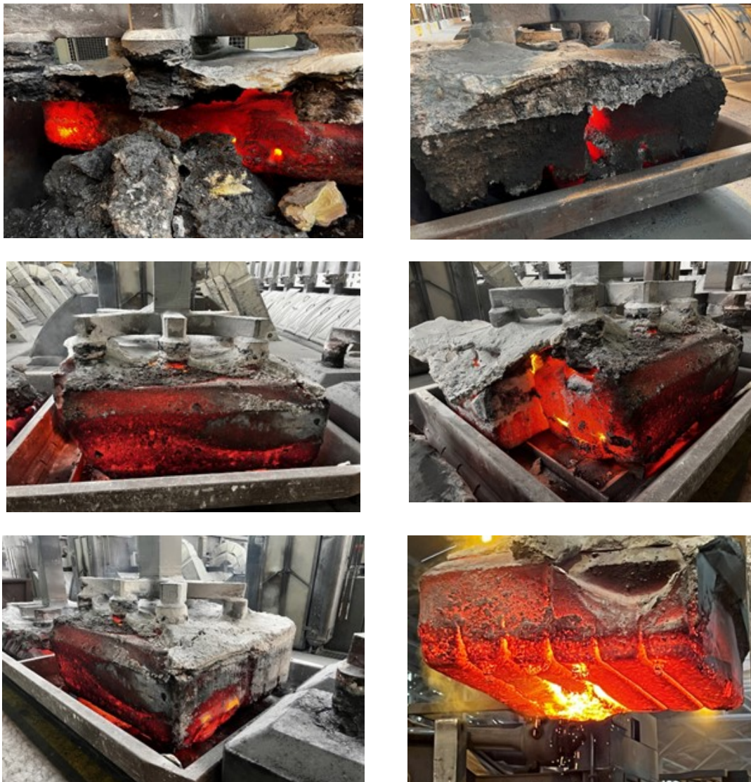
Figure 2. Type of anodic incidents and fallen blocks.
